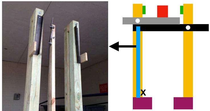
In the loaded configuration (**diagram**), the counterweight end of the throwing arm (red), rests on top of the compound lever system formed by the angle irons. The lower piece of angle is propped in place by a piece of wood (blue). A rope attached approximately at the position shown with the arrow is pulled to activate the release. You may need a small block of wood or similar (X) at the bottom of the prop to prevent it from kicking back into the tower gap when the shot is triggered.
