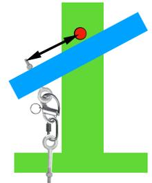
A system utilizing a shackle of this nature will be approved as long as the remainder of the release is deemed safe. Both ends of the snap shackle assembly must be anchored with a through bolt (has the nut on the opposite side relative to the direction of pull). A release that attaches to the machine using hardware similar to the hasp staple shown here, which is held to the arm or frame using screws, **will not be approved**.
